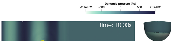
Fig. 19. Screen shots of the dynamic pressure field across the domain (left), and on the WEC body (right) for sea state MS04. The black line on the WEC hull indicates the instantaneous free surface.
