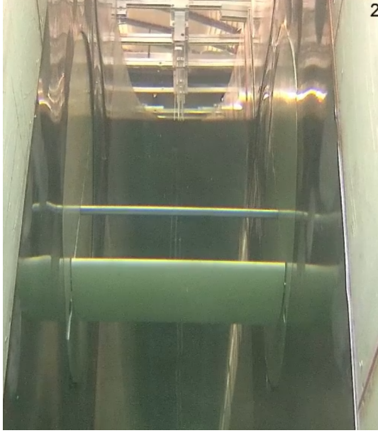
Fig. 3: Rotor with fairings in a sub-canal (Photo of the experiment)
